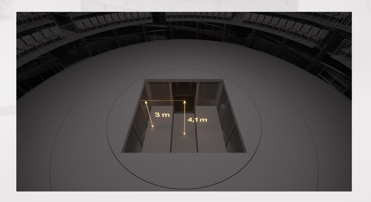
There is a flybar system on three concentrical girders on which chain or rope hoists are mounted. Hoist positions can be pre-adjusted by moving hoist motors. Flybar system is computer controlled with precision control and weight measuring system.
